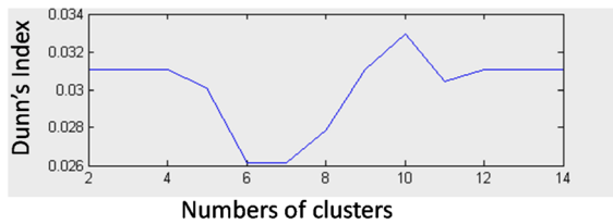
Fig. 5 Dunn's Index calculates the compactness and separateness of clusters. The highest index score suggests ten clusters as an optimal number of hidden cognitive states
