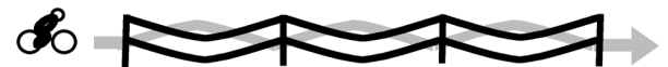
Figure 2. Schematic of actual and visually experienced paths followed by a cyclist riding behind curved rails.
